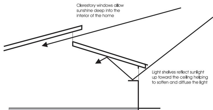
A light monitor is another way to enhance daylighting. A light monitor is essentially a box mounted on top of the roof with a window facing either south or north. A south-facing window would be shaded by the overhang to block direct sunshine during the summer. Like a clerestory window, sunlight enters the light monitor and is reflected down into the room below. Light diffusing shades are sometimes used with a
