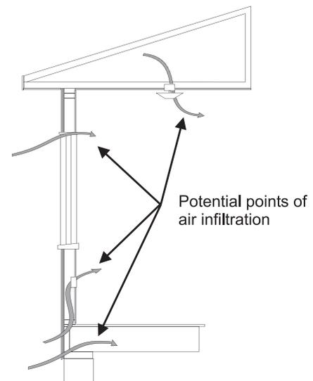
there are fewer areas for potential air infiltration compared to frame construction, further improving energy efficiency.
